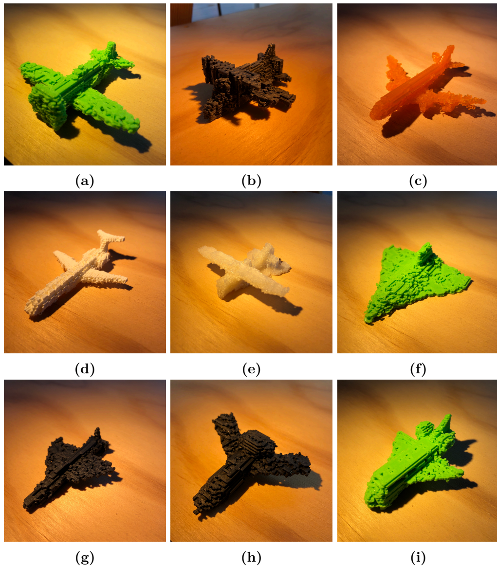
Figure 7.11: Nine examples of 3D printed STL files exported from the DeepIE3D web application. The colors are arbitrary and has no meaning. (a), (c), (f) and (i) are printed on an Ultimaker 2 Extended; (b), (g) and (h) are printed on an Ultimaker 2+; and (d) and (e) are printed on a Makerbot Replicator
